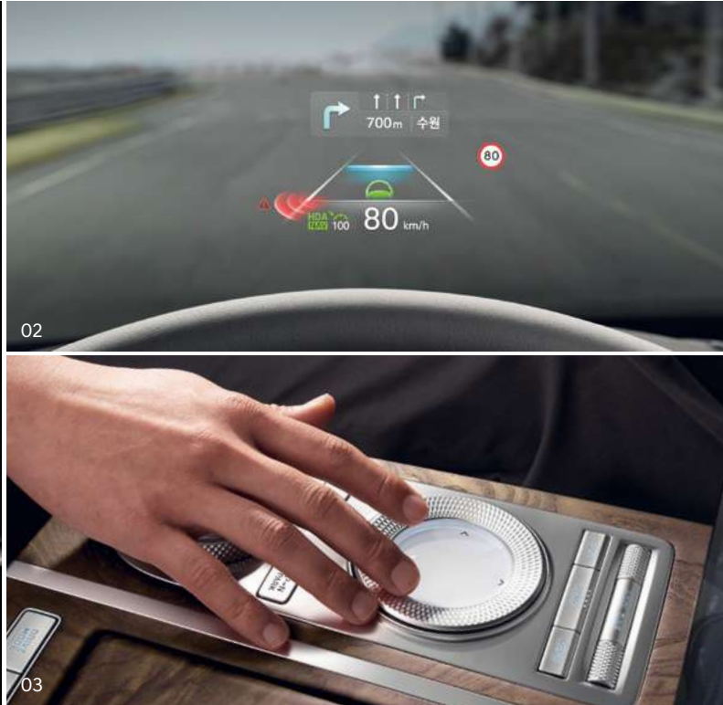
02. Head-Up Display _ Shows driving speed and GPS information, as well as key driver assist information and crossroads. The high-resolution, 12" wide display boasts clear visibility during daytime or nighttime. 03. GENESIS touch controller _ Located on the center console, this allows users to control the various infotainment systems easily without having to repeatedly touch any buttons or screens. Its handwriting recognition system helps users set a destination or enter a phone number simply by using handwritings instead of typing into a keyboard.
