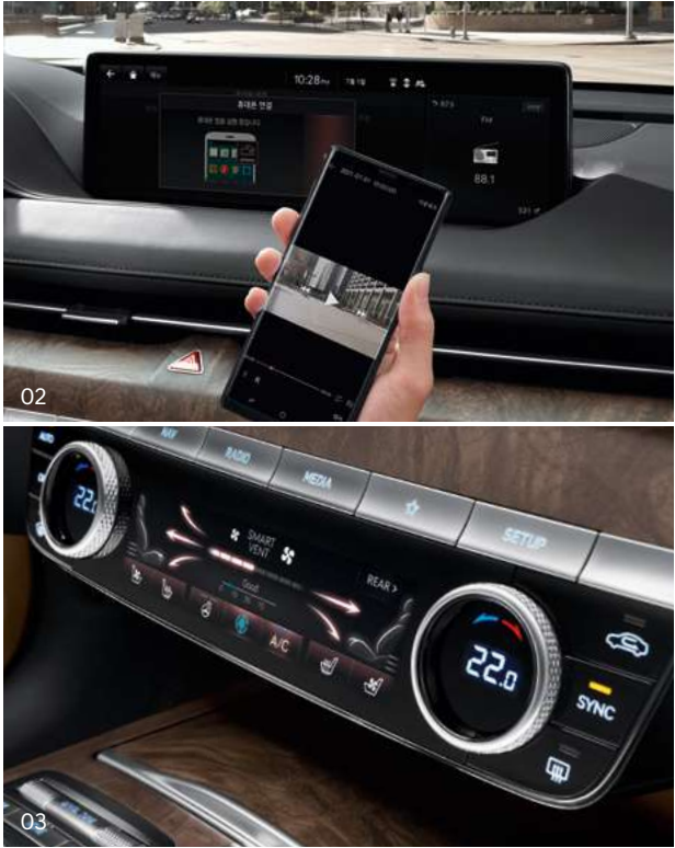
02. 03. Built-in camera _ Cameras on the front and rear ends of the vehicle allow users to see video images live or save them to playback/download, or upload to social media outlets via the vehicle's display screen or a smartphone. Touch-type climate control panel (including haptic feedback) _ This system can control air conditioning/heating for front and rear seats. It also features an air purification system that dramatically reduces the level of fine-dust in the vehicle.
