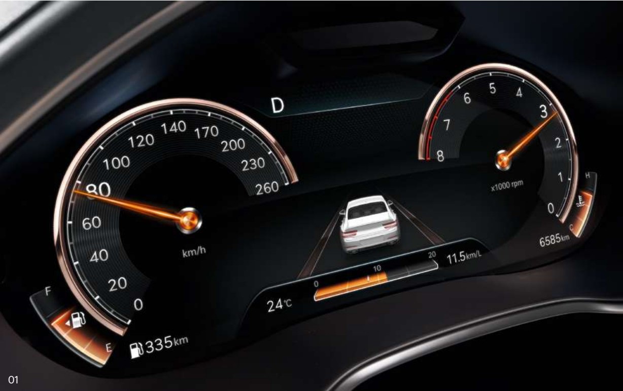
01. 12.3" 3D cluster _ The wide, high-resolution 12.3" 3D cluster provides various view modes and differentiated drive mode illumination. The cluster's embedded camera tracks the driver's eye movements to provide 3D information at any angle, maximizing visibility.
