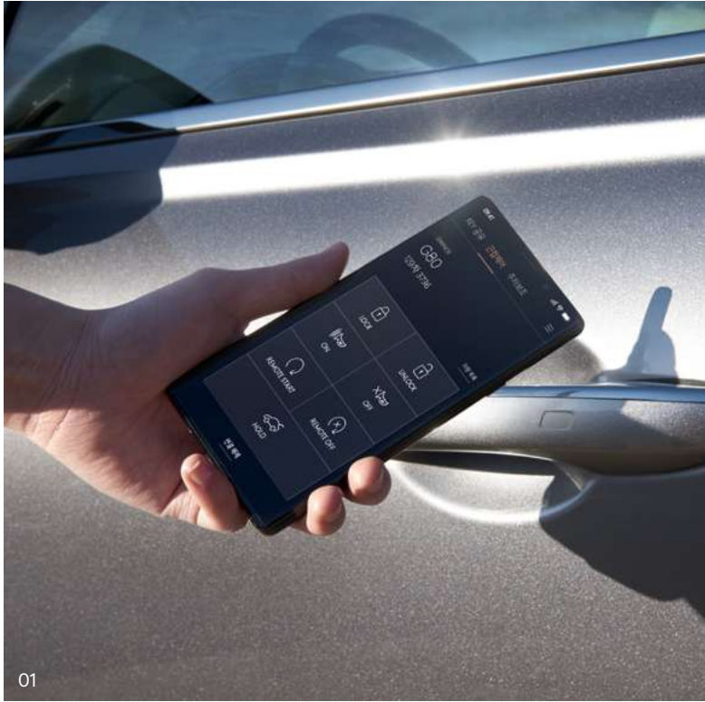
01. GENESIS digital key _ Users can lock and unlock their vehicle by simply touching the door handles with a smartphone downloaded with the digital key app, or start the engine with the smartphone placed on the console's wireless charging pad. The digital key can be shared by friends and family and also be used to control selected vehicle systems from a remote distance of approximately 10 meters.
