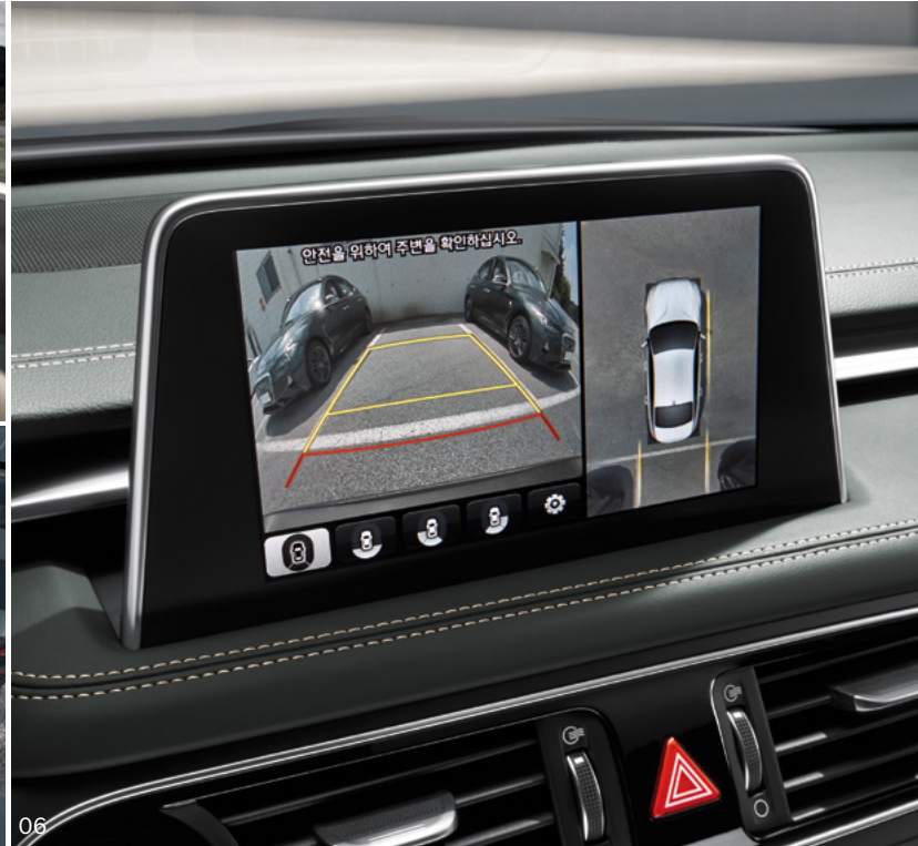
06. Surround View Monitor (SVM) system _ 4 HD cameras mounted on the front, sides, and rear of the vehicle show the surroundings in real time. Markings on the video image show distance from obstacles in the front and the back, and video projections of the back show the vehicle's anticipated trajectory when moving in reverse.
