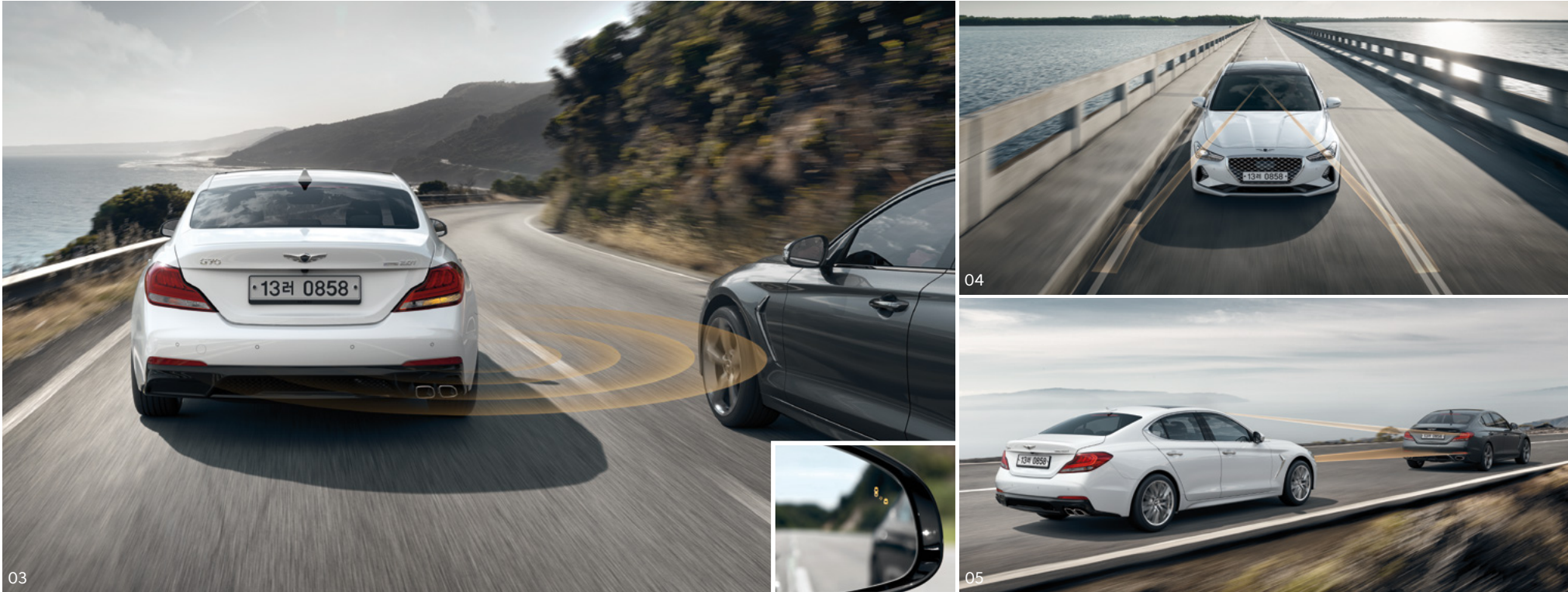
03. Blind-Spot Collision Warning (BCW) system _ Two radars installed on the rear of the vehicle detect and warn the driver of fast-approaching vehicles in blind spots or on the side of the back of the car.
