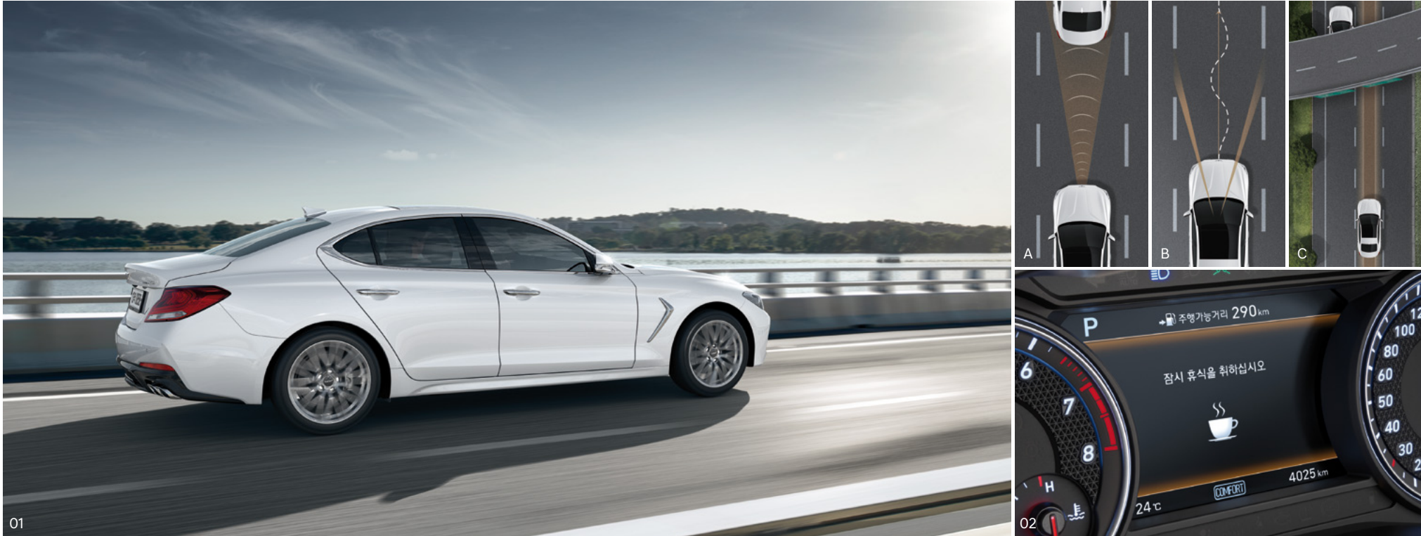
01. Highway Driving Assist (HDA) system _ An automated system helps control the speed of the car and keep the vehicle in the lane while driving on the highway by using comprehensive information such as distance from the car ahead, lanes, and navigation-based speed limit, eliminating the need to step on the brakes or the accelerator during long distance travel or while driving through congestion. A. Longitudinal (headway distance) control B. Lateral (lane keeping) control C. Highway-specific control
