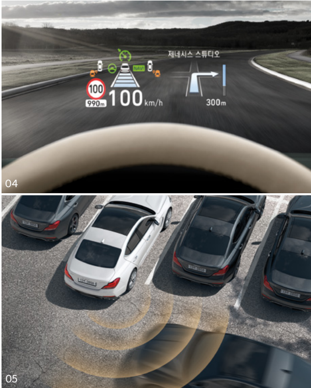
04 & 05. Head-Up Display (HUD) _ Vehicle information is projected on the front windshield through an 8" image with optimized brightness for excellent visibility even during the day. Rear Cross-Traffic Collision Warning (RCCW) system _ Warns the driver of cross-traffic approaching the vehicle from the back while pulling out in reverse.
