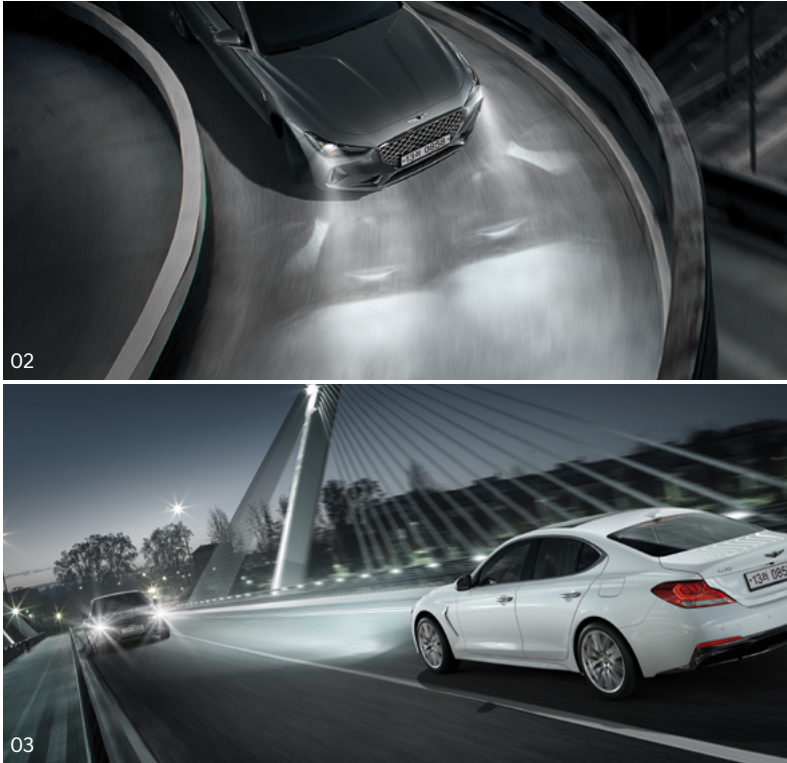
02. Low Beam Assist-Dynamic (LBA-D) system _ Headlamps steer automatically to the left or the right together with the steering wheel, improving visibility and reducing blind spots while driving at night. 03. High Beam Assist (HBA) system _ Sensor monitors headlamps of oncoming (or tail lamps of preceding) vehicles and brightness of surroundings to switch between high beam and low beam automatically, promoting the safety of the driver as well as oncoming (or preceding) vehicles while driving at night.
