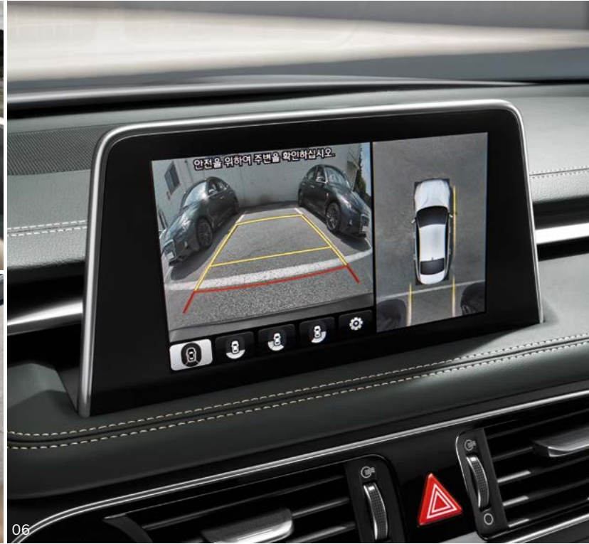
06. Surround view monitor _ 4 HD cameras mounted on the front, sides, and rear of the vehicle show the surroundings in real time. Markings on the video image show distance from obstacles in the front and the back, and video projections of the back show the vehicle's anticipated trajectory when moving in reverse.
