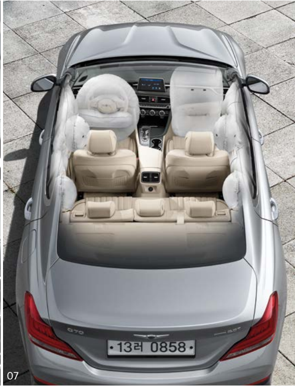
07. 9-airbag system _ Advanced airbags in the driver and front seats regulate the degree of inflation and timing of deployment according to the occupant's weight, position, and force of collision. 9airbags, including a driver's knee airbag, front and rear side airbags, and curtain airbags, minimize injuries.
