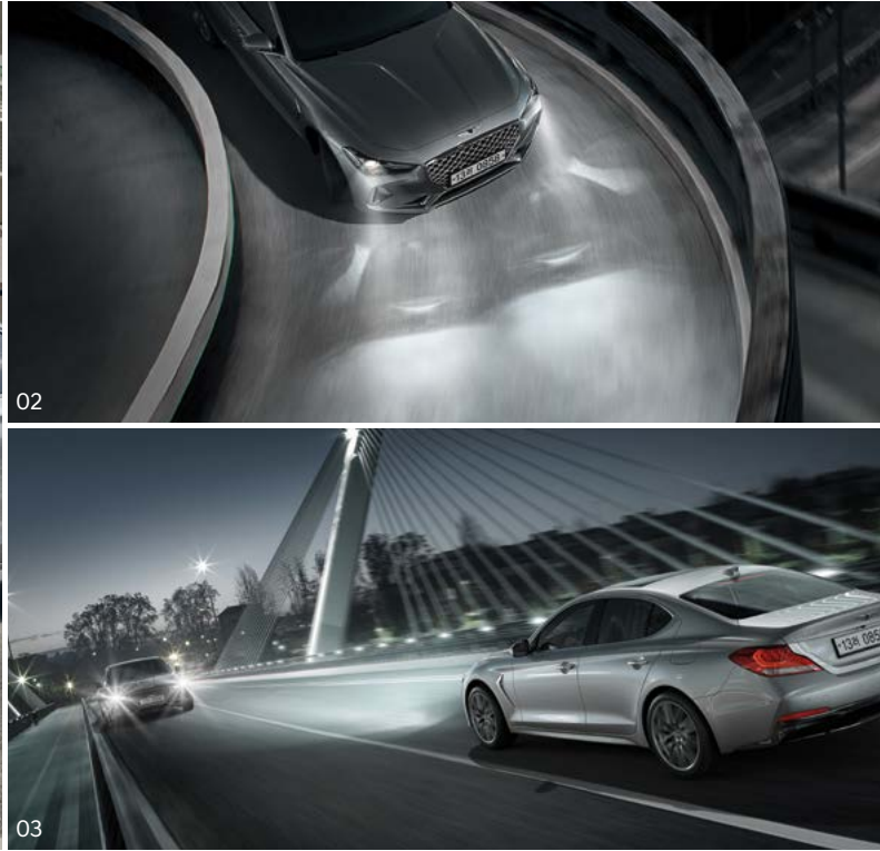
02. Low beam assist-dynamic (LBA-D) _ Headlamps steer automatically to the left or the right together with the steering wheel, improving visibility and reducing blind spots while driving at night. 03. High beam assist (HBA) _ Sensor monitors headlamps of oncoming (or tail lamps of preceding) vehicles and brightness of surroundings to switch between high beam and low beam automatically, promoting the safety of the driver as well as oncoming (or preceding) vehicles while driving at night.
