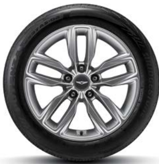
225/50R17 Bridgestone tires & wheels (basic specification for 2.2D)
