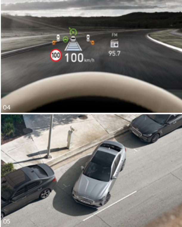
04 & 05. Head-up display (HUD) _ Vehicle information is projected on the front windshield through an 8" image with optimized brightness for excellent visibility even during the day. Parking distance warning (PDW F/R) _ Sensors mounted on the front and rear of the vehicle track distance from obstacles and sound an alarm to assist drivers while parking.
