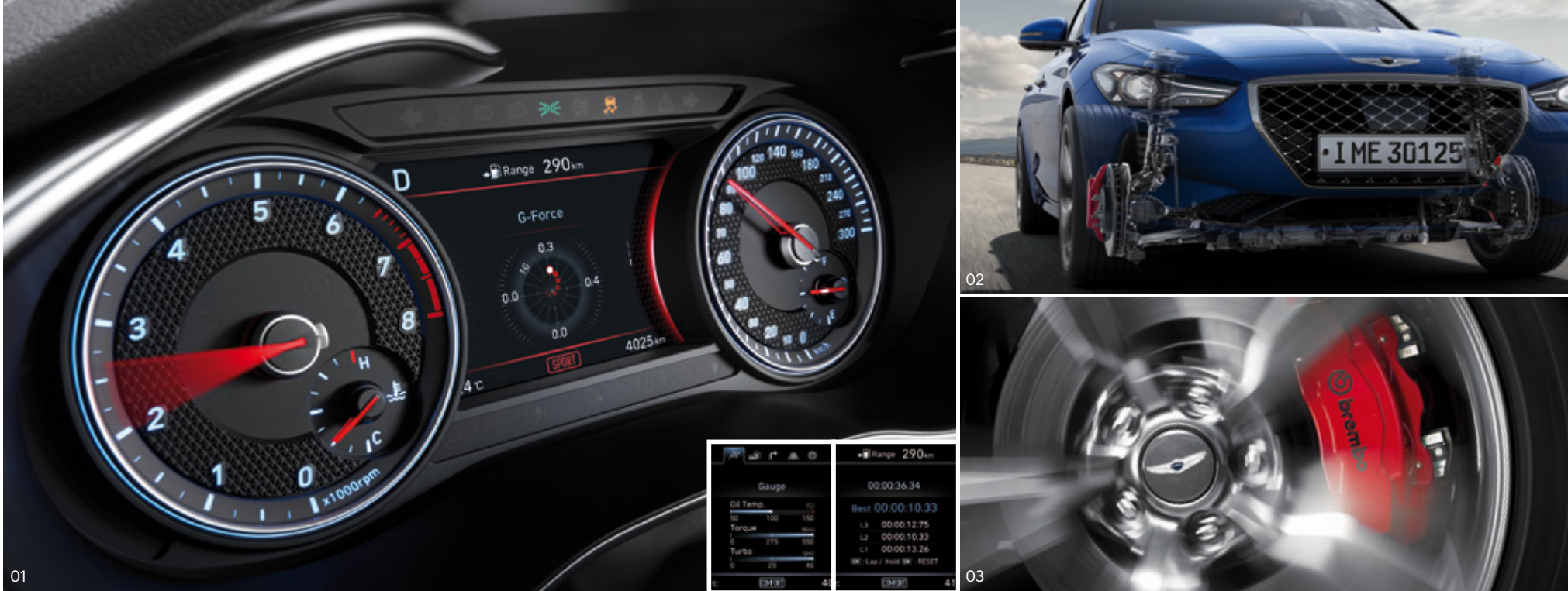
01. 7" TFT LCD cluster _ The engine oil temperature gauge, torque gauge, turbo booster gauge, lap timer (shows the best and the 3 most recent lap times), and G-Force (shows the current top, bottom, left, and right gravity acceleration or G values) can be seen through the cluster which also amplifies the enjoyment of high-performance driving with differentiated content.
