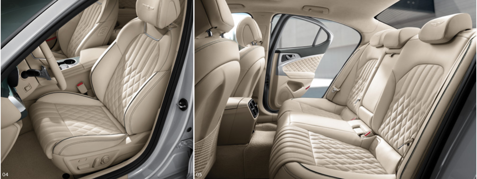
04. Intelligent driver's seat _ An 8-way power seat, 4-way power lumbar support, 2-way power bolster, and 2-way electric cushion extension optimize seat adjustments to conform to the driver's body and posture and maximize comfort. Seat positions are displayed on the AVN screen for more convenient operation.
