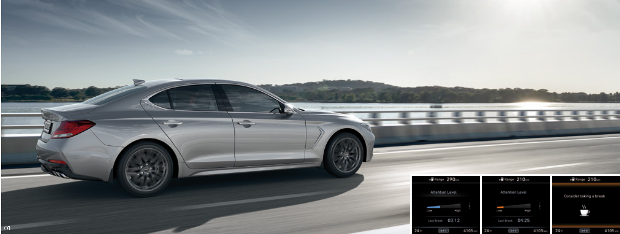
01. Driver attention warning (DAW) _ A comprehensive system analyzes driving patterns of the driver and the vehicle's position in the lane to operate a 5-stage warning system. It posts pop-up messages and sets off warning signals to encourage the driver to rest when it detects driver fatigue or inattentive driving.
