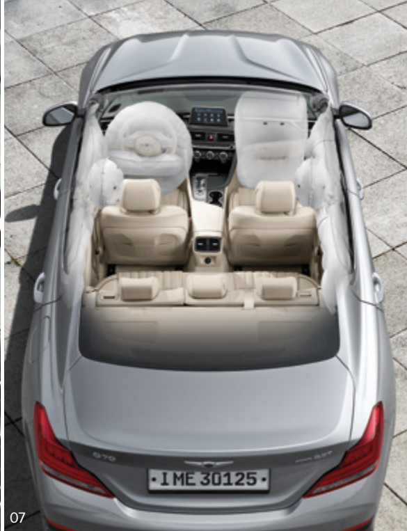
07. 7-airbag system _ To help protect occupants and potentially reduce injuries in the event of a collision, front passenger airbags, two front-side airbags, two side-curtain airbags, and a driver's knee airbag are offered as standard. The driver's knee airbag is designed to minimize impact and injury to the driver's lower extremities in the event of a collision.
