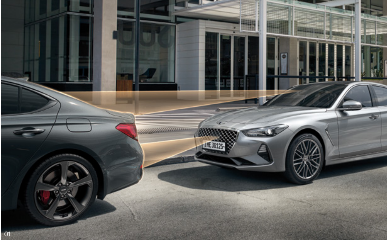
01. Forward collision-avoidance assist (FCA) _ Comprehensive monitoring of front radar and camera signals warns the driver of potential forward collisions, applying the brakes if warranted. It is a high-tech preventive safety system that even takes into consideration the safety of other vehicles.
