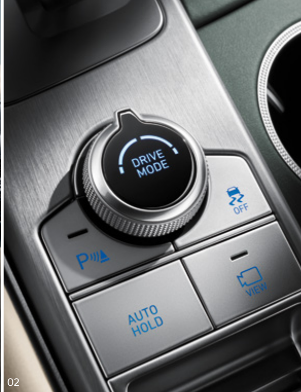
02. Drive mode control system _ Drivers can switch between Comfort, Eco, Sport, Smart, or Custom driving modes according to personal preference or driving situation. G70 offers exceptional driving and riding comfort by optimizing power distribution for each driving mode.
