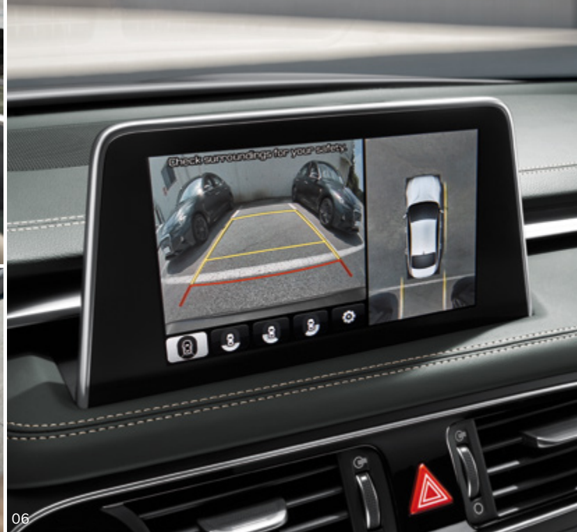
06. Around view monitor (AVM) _ 4 HD cameras mounted on the front, sides, and rear of the vehicle show the surroundings in real time through the AVN screen. Markings on the video show distance from obstacles in the front and the back, and video projections of the back show the vehicle's anticipated trajectory while moving in reverse.
