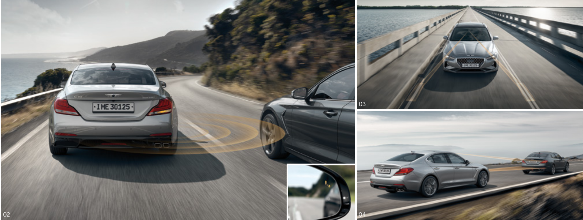
02. Blind-spot collision warning (BCW) _ Two radars installed on the rear of the vehicle detect and warn the driver of fast-approaching vehicles in blind spots or on the side of the back of the car.
