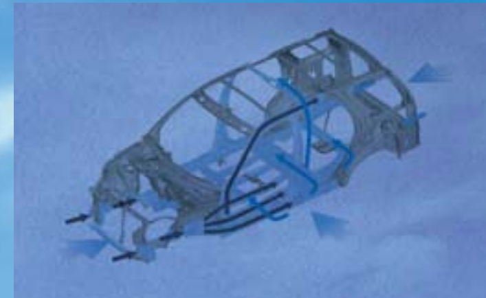
Body structure is designed to protect front and rear passengers in the event of impact.
