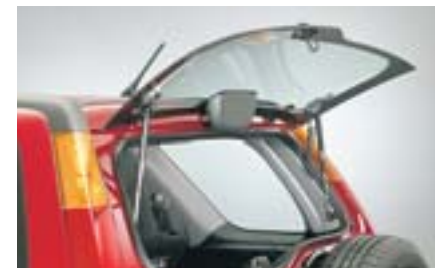
Side hinged, 2 way tailgate for easy access
