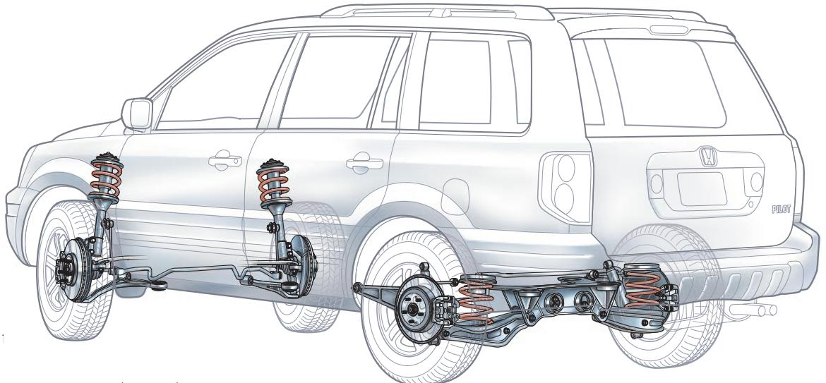
**Become more independent.** When the road gets rough, that's where the virtues of the Pilot's 4-wheel independent suspension really shine. This tough, yet very refined, **front strut and rear multi-link suspension** takes what the road dishes out in stride, whether paved or unpaved, while still providing a smooth, car-like ride with excellent handling. And its wide track is designed to provide an extra measure of stability.
