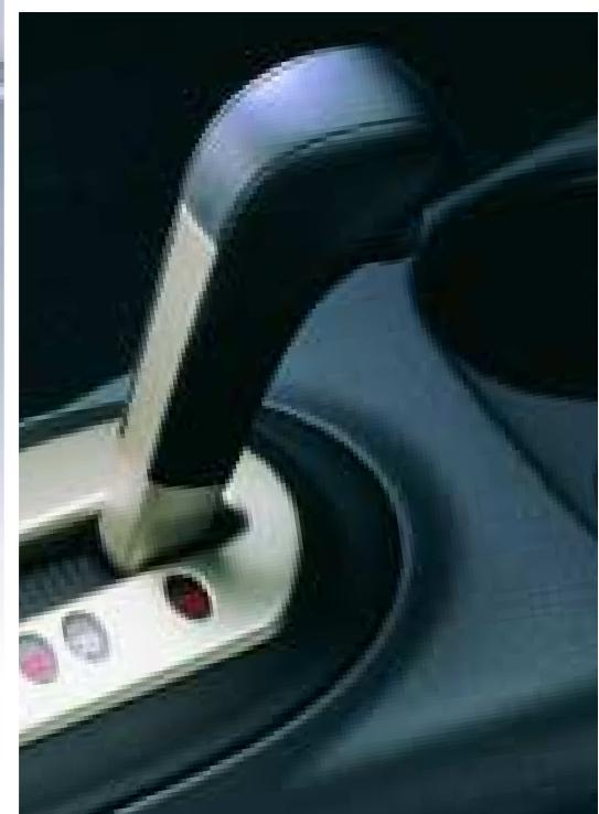
The Civic Sedan features Honda's Continuously Variable Transmission. This CVT is smaller, lighter and more efficient than any conventional automatic. It uses a dynamic pulley system to offer an infinite range of gear ratios, giving you remarkably seamless operation. You'll never feel it change gear and the engine can operate at maximum efficiency at all times.
