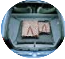
Luggage net - To reduce the movement of luggage and goods whilst travelling. Simple to install and remove.
