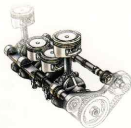
Accord 4-cylinder engines have a Honda-designed second order balance system that uses dual counter-rotating shafts to help reduce engine vibrations. This reduces vibration transmitted to the cabin, resulting in a quieter ride.
