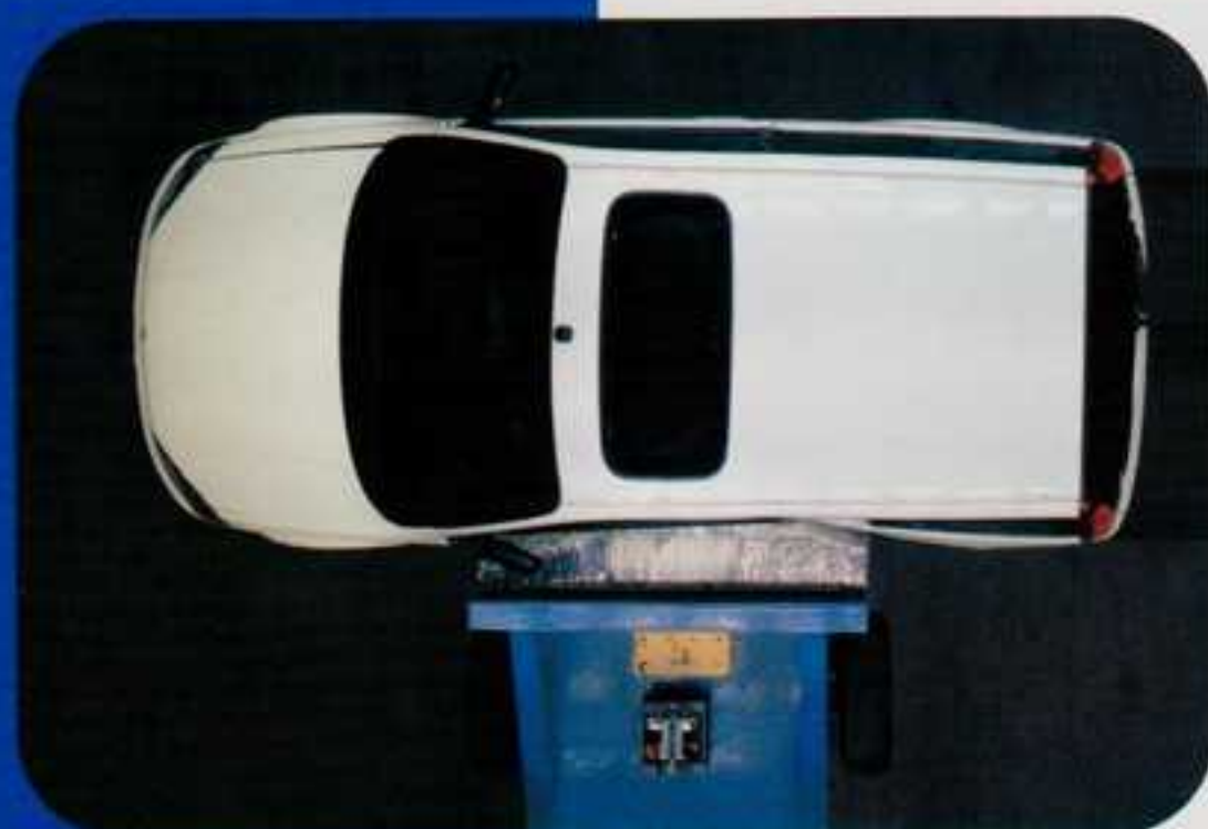
Side impact crash test
