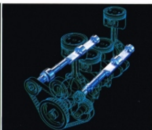
Two secondary balancer shafts built into the Accord's aluminium engine block reduce vibration and noise created by engine rotation at mid to high RPMs.
