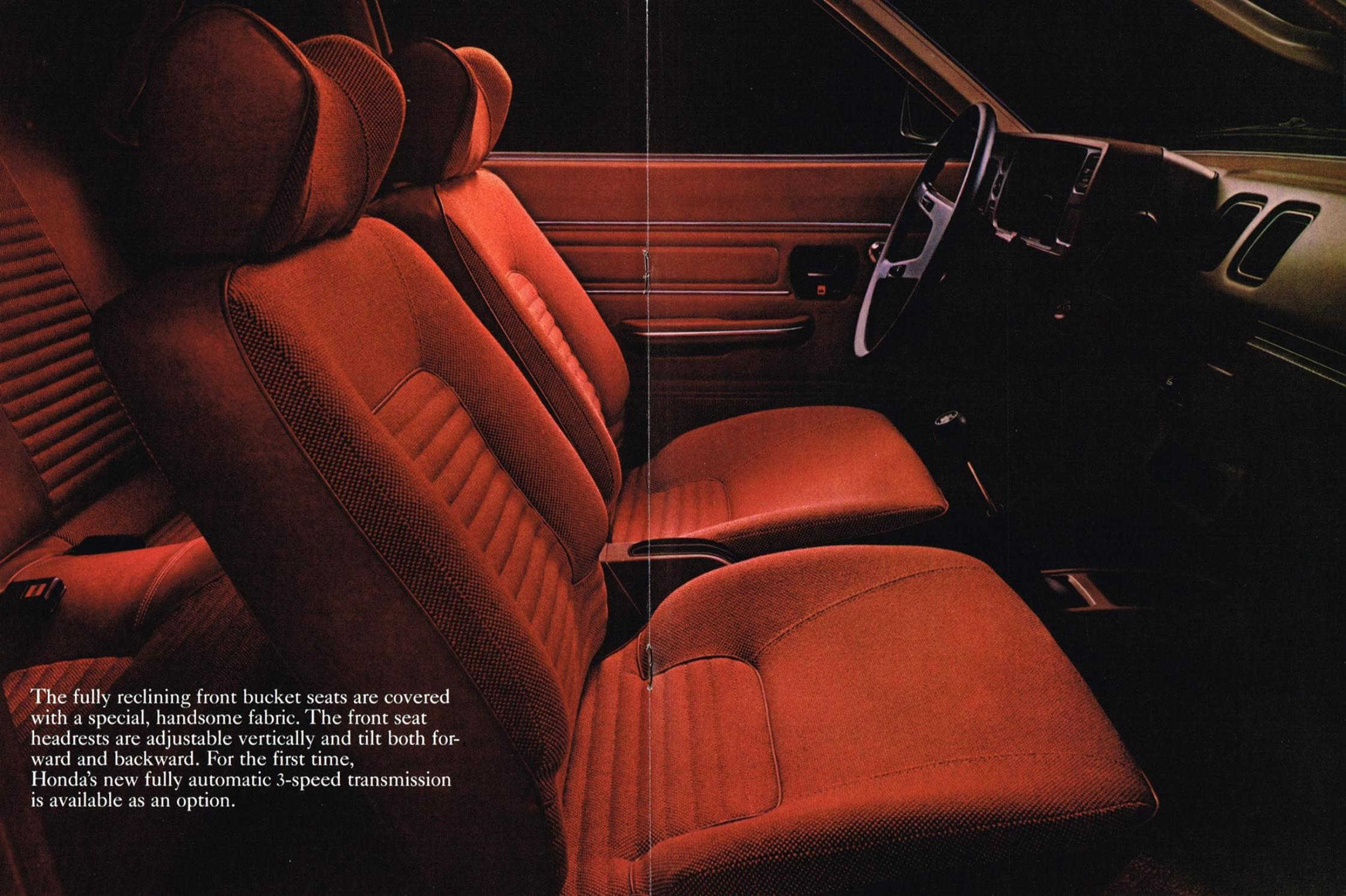
The fully reclining front bucket seats are covered with a special, handsome fabric. The front seat headrests are adjustable vertically and tilt both forward and backward. For the first time, Honda's new fully automatic 3-speed transmission is available as an option.
