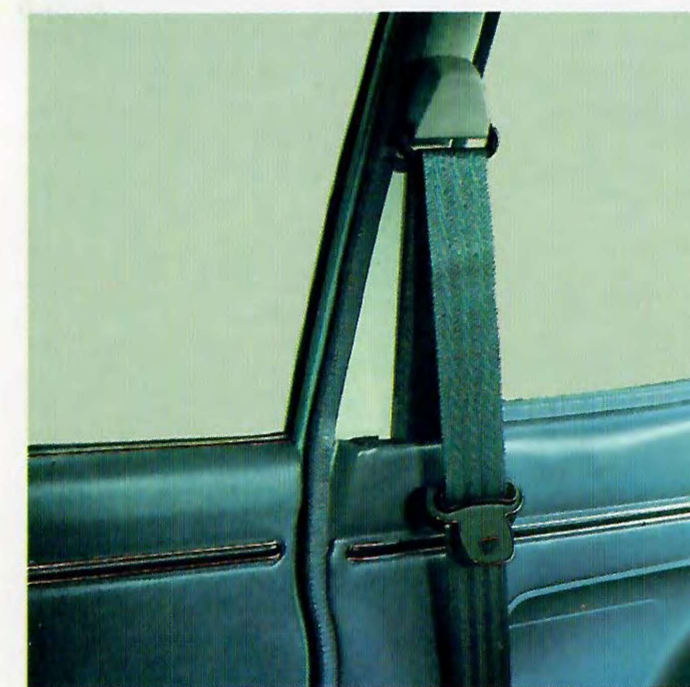
Both models of the Accord are designed so that the front seatbelts retract into the body side panel. This keeps the belts out of the way to make it easier for passengers to enter or leave the rear compartment.
