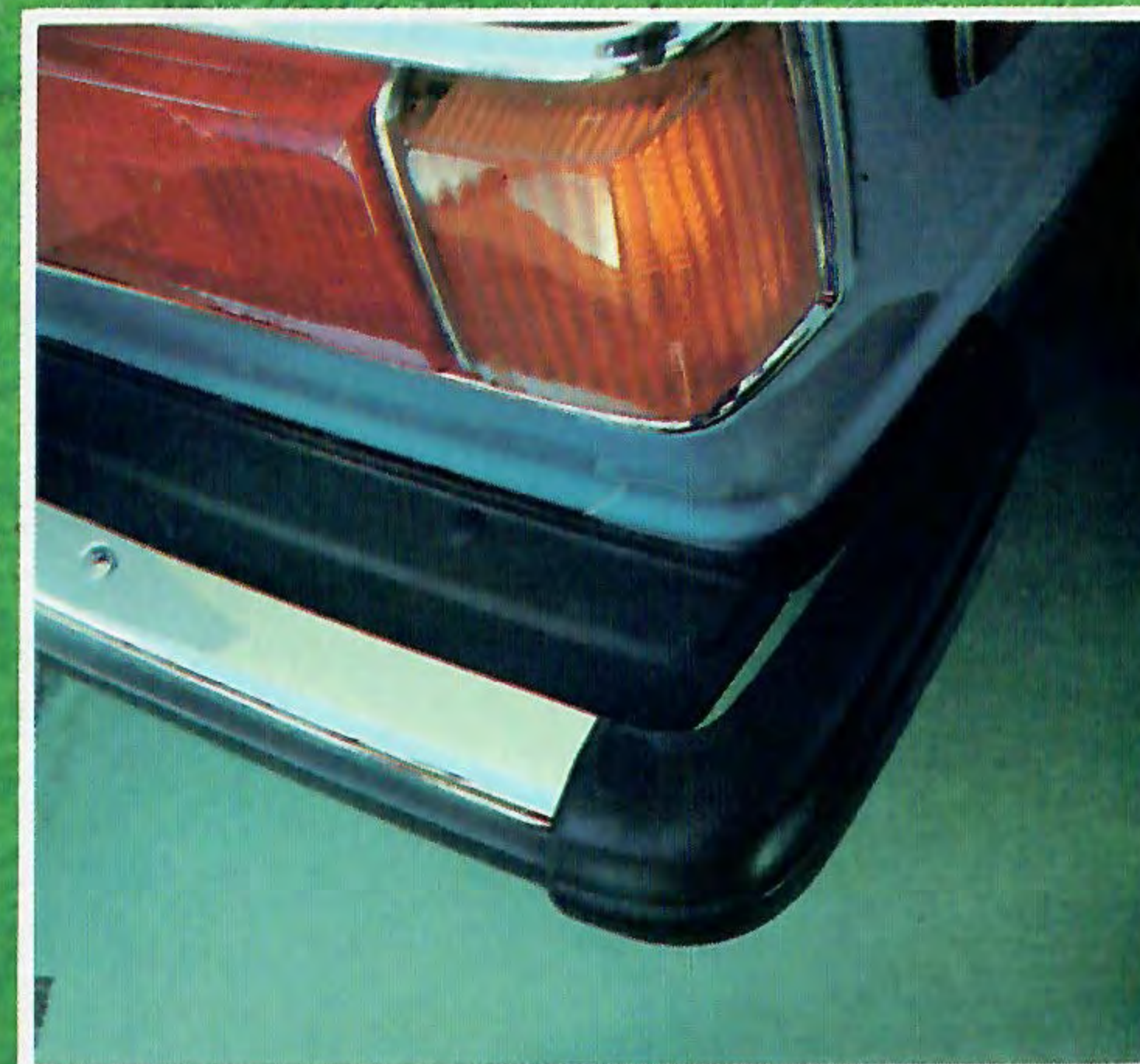
The energy-absorbing bumpers on the Accord have been redesigned for 1978. Notice the added protection provided by the new bumper end extensions.
