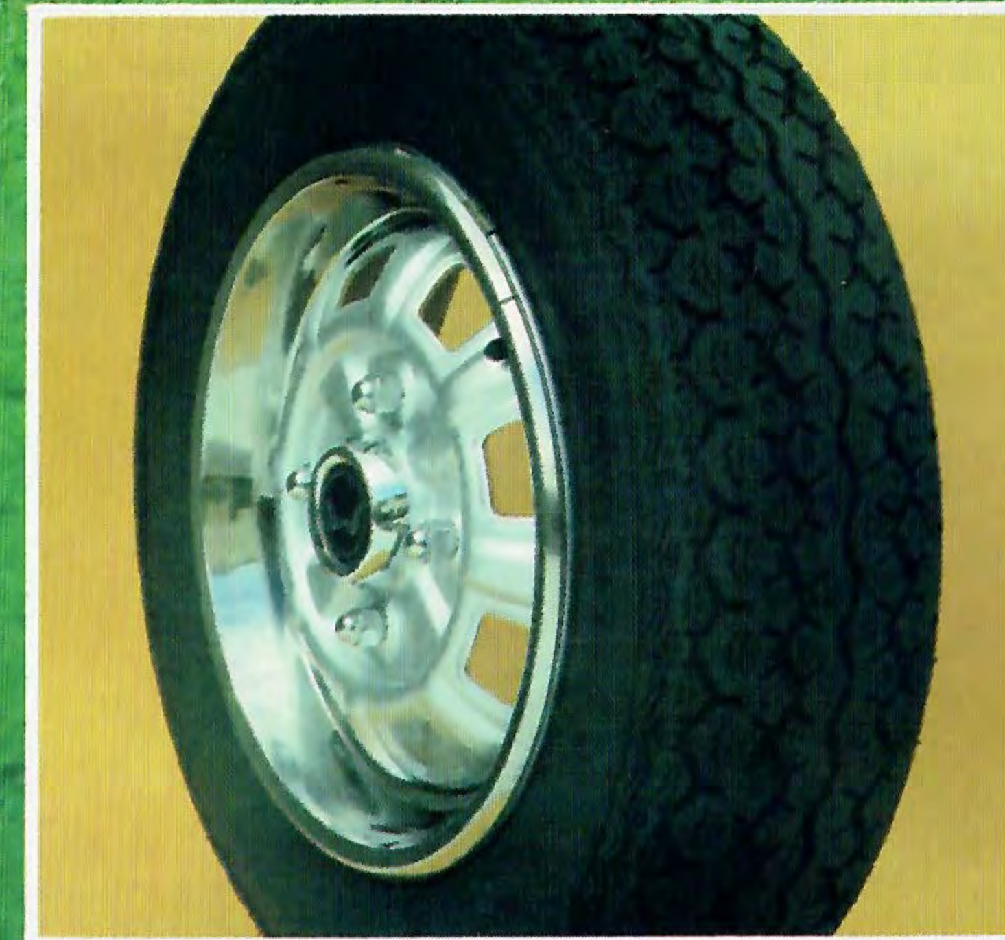
The Accord comes equipped with radial ply tires. Radial tires improve the ride and handling and also improve overall fuel economy because of less rolling resistance. Trim rings are standard.
