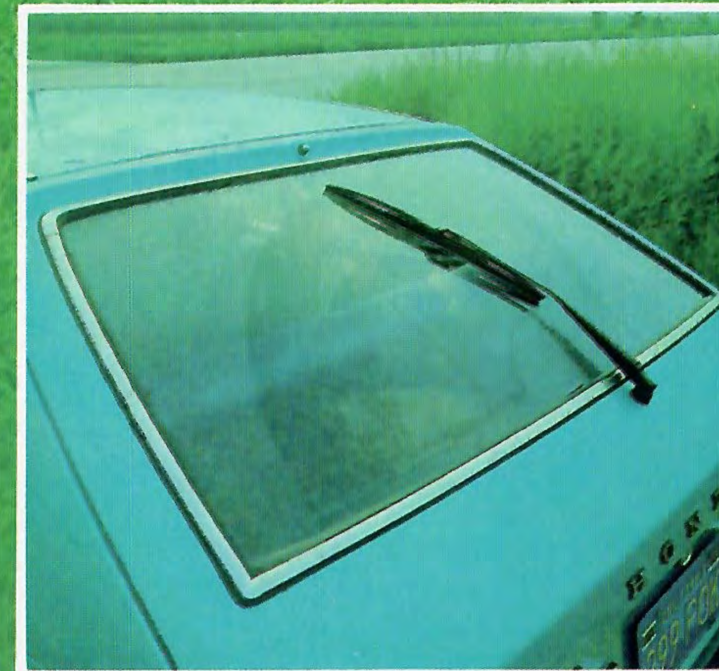
Both Accords are equipped with a rear window washer and wiper to help keep the window clean under severe driving conditions. A rear window defroster is also standard.
