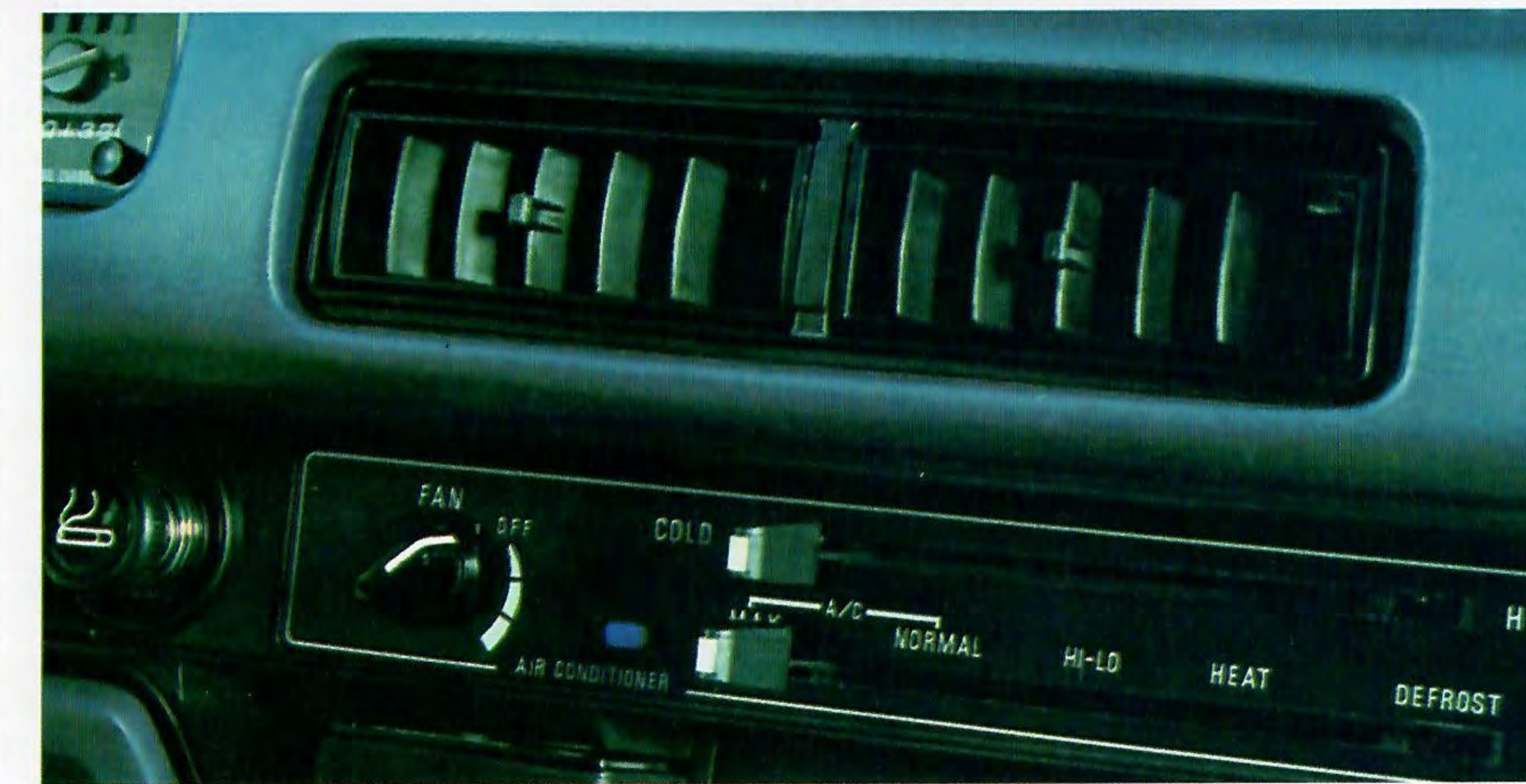
Optional air conditioning unit designed for the Accord fits right into the standard heater/ventilation system. Air outlets are positioned to provide maximum circulation of cooled air without causing annoying drafts.
