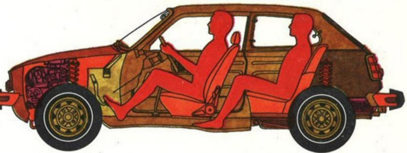
To give you this space the engine was mounted transversely—sideways—so it doesn't intrude on the leg room in the passenger compartment.
