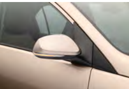
ORVM with Electric Adjustment & Turn Indicators
