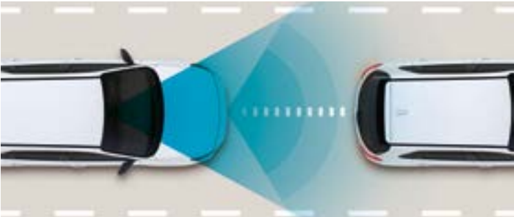
Autonomous Emergency Braking (AEB). Automatically applies partial or maximum braking force if a potential collision is detected.
