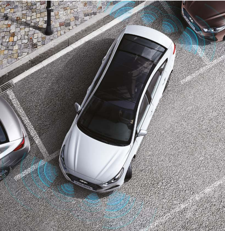
Parking Assist System (PAS) Assists the driver during reverse movement of the vehicle by activating an audible warning if you get too close to objects.
