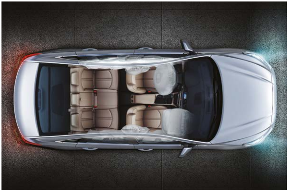
Blind Spot Detection (BSD) Detects approaching vehicles or unforeseen objects in the blind spot and triggers a warning light and acoustic alert when changing lanes. 6-Airbag system Comprises dual front airbags, two side impact airbags at the front and two curtain airbags running the length of the cabin.
