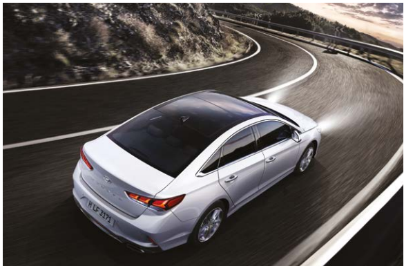
Advanced Smart Cruise Control (ASCC) Maintains a constant speed and distance from the vehicle ahead by automatically accelerating and braking by using a front radar sensor. Dynamic Bending Lights (DBL) Respond to the turn of the steering wheel and illuminate the part of the road you're turning towards for safer driving at night.
