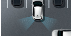
Rear Cross-Traffic Collision Warning (RCCW)
