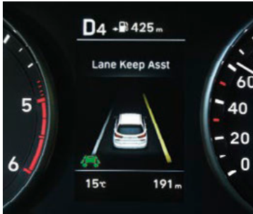
Lane Keep Assist System (LKAS) recognises lane markings and can apply corrective steering through long motorway journeys.
