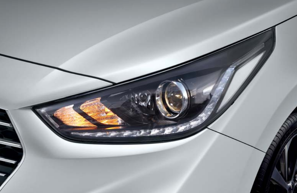
Projection headlamps with LED position & DRL lamps
