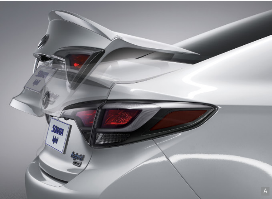
A. Smart trunk system The trunk opens automatically by sensing your presence with the smart key—there's no need to press any button. Perfect when your arms are full and when carrying heavy loads.
