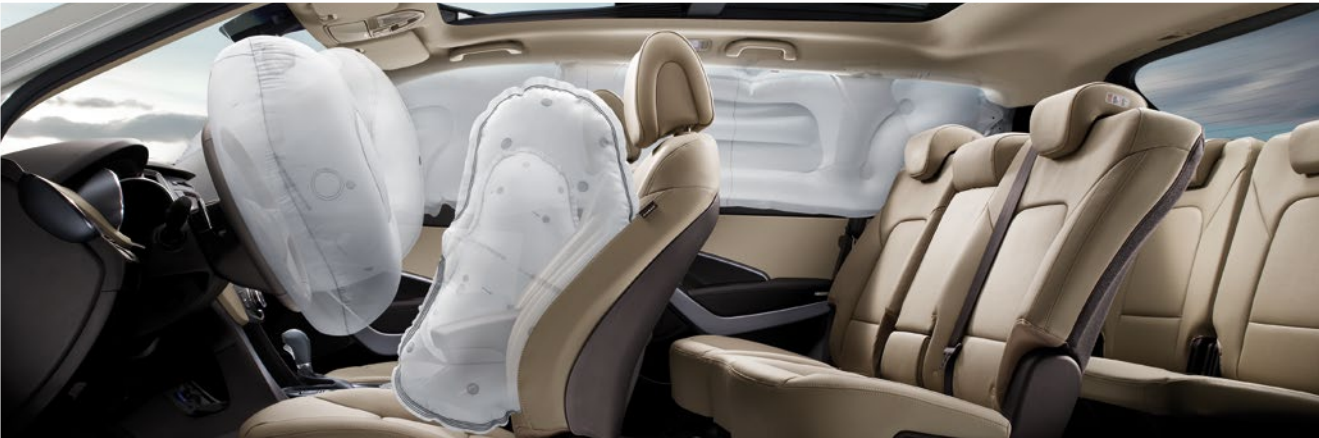
6-airbag system Santa Fe is equipped with front airbags, 2-side airbags, and curtain airbags that minimize passenger injuries in the event of a collision.
