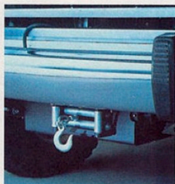
Hidden winch (dealer installed)
