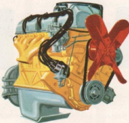
**'JEEP' TORNADO-OHC ENGINE.** There aren't many engines that can keep you moving at freeway speeds and still provide enough power for traction over the rugged routes. With its exclusive overhead cam design, Tufftridized crankshaft, spheroidal combustion chambers, ventilated crankcase and extra large valves, the TORNADO-OHC has yet to be matched by any automotive manufacturer. It's the powerful good friend of every 'Jeep' Gladiator owner.
