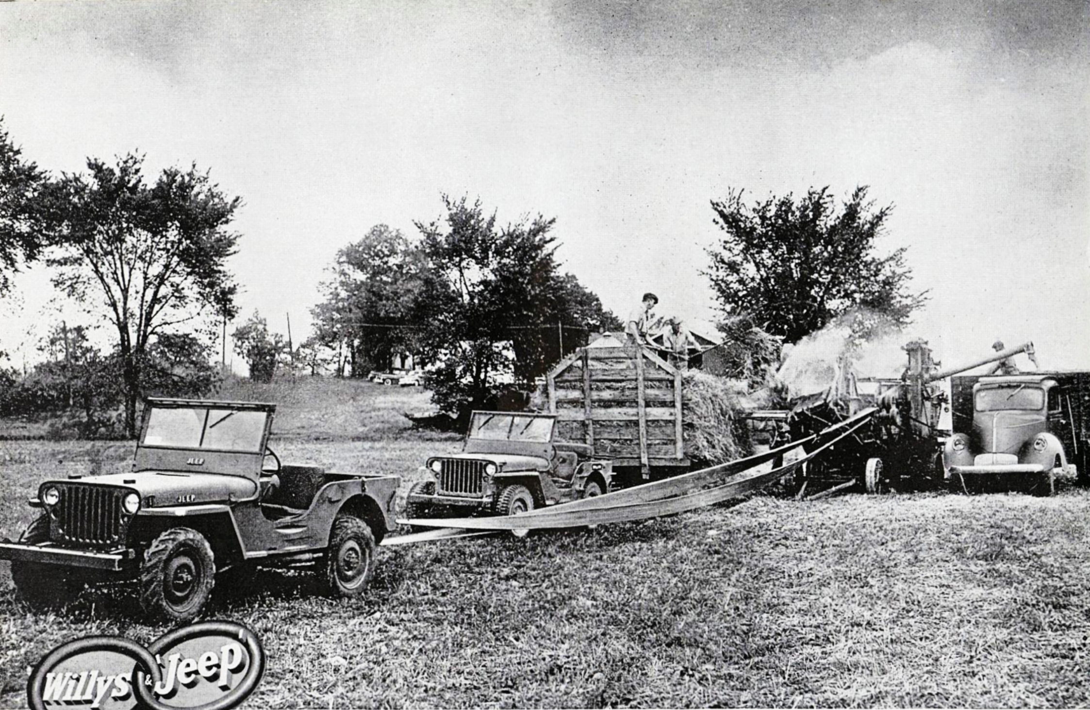
THRESHING . . . Here's the familiar threshing job showing the Universal "Jeep" feeding plenty of power to the separator. With Jeep power it threshed 197 bushels of oats out of this field in one hour. Gas used by the Jeep—under 2½ gallons.
