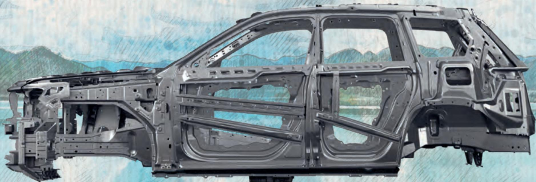
**STRONG AND LIGHTWEIGHT** The exceptionally solid safety cage consists of high-strength steel paired with lightweight aluminum, designed to make Jeep® Grand Cherokee light in weight while still providing a very strong foundation. Standard.
