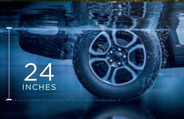
Use your available Quadra-Lift® Air Suspension System to raise Jeep® Grand Cherokee 4xe to its highest level of ground clearance. You're then able to confidently travel in up to 24 inches of water.<sup>6</sup> Grand Cherokee 4xe is engineered to take water fording<sup>6</sup> seriously, thanks to the placement and waterproofing of critical functions.
