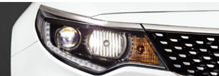
Single Projection-type Headlamps with LED DRLs (LX)
