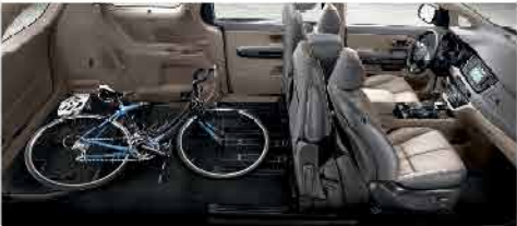
UNIQUE SLIDE-N-STOW SEAT DESIGN. When you need more cargo area, you can take advantage of the available 10 second-row seats' innovative stand-up design. Simply flip a lever to stand the seats upright, where they stay locked in place. Third-row seats conveniently fold down into the floor, and they also feature a versatile 60:40 split-fold design, giving you the option of carrying a combination of passengers and cargo.
