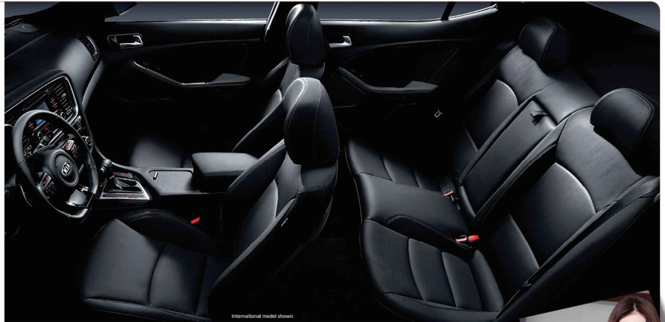
HEATED AND COOLED SEATS. Standard heated front seats and available heated rear seat cushions help ensure comfortable driving in cold weather. Enjoy optimal comfort in warm weather with available air-cooled driver and front passenger seats that circulate air through perforations in the seat leather.
