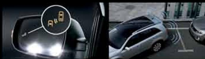
**BLIND SPOT DETECTION (BSD).<sup>1</sup>** BSD uses radar sensors in the rear bumper of the vehicle to detect vehicles you may not be able to see because they're in your "blind spot". When the system identifies a vehicle in a blind spot, it activates a warning light in the side mirror to warn you. If the vehicle is present when you signal for a lane change, an audible alarm sounds to help you avoid a possible collision.
