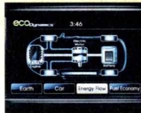
POWER RATIO GAUGE The power ratio gauge lets you know when the vehicle is operating with the electric motor, with the gas engine, or with both. It also provides information about the regenerative battery-charging system and is standard on Optima Hybrid Premium.
