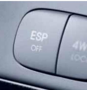
◀ **ELECTRONIC STABILITY PROGRAM (ESP) WITH TRACTION CONTROL SYSTEM (TCS).** THESE STANDARD, ADVANCED, ACTIVE SAFETY FEATURES ARE IN PLACE FOR ADDED SECURITY. TCS OFFERS IMPROVED TRACTION BY DETECTING AND CORRECTING WHEEL SPIN, WHILE ESP GIVES YOU IMPROVED DIRECTIONAL STABILITY TO HELP YOU MAINTAIN CONTROL IN THE EVENT OF A SEVERE SKID.
