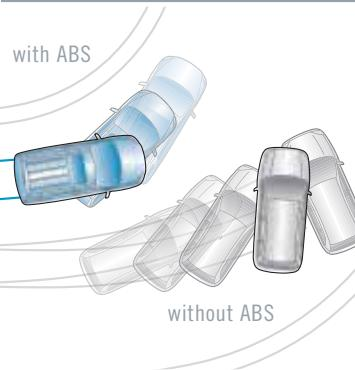
▲ **STANDARD ANTI-LOCK BRAKES** PROVIDE BETTER VEHICLE CONTROL WHEN STOPPING IN DIFFICULT CONDITIONS LIKE WET OR SLICK ROADS. SENSORS MONITOR EACH WHEEL, AND IF ONE IS ON THE VERGE OF LOCKING, THE BRAKES ARE PUMPED. THIS HELPS YOU MAINTAIN THE ABILITY TO STEER DURING HARD BRAKING AND GIVES YOU GREATER CONTROL IN AN EMERGENCY.
