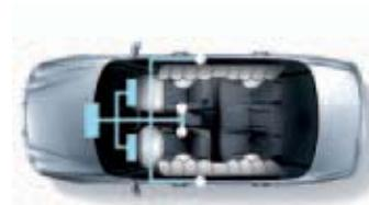
► **AIRBAG SENSORS.** THE AMANTI'S COMPUTER-CONTROLLED AIRBAGS ARE ASSISTED BY SENSORS THAT WORK IN CONJUNCTION WITH THE SEAT-BELT SENSORS. BEFORE THE AIRBAGS WILL DEPLOY, THESE SENSORS GAUGE THE SEVERITY OF A FRONTAL IMPACT. THIS ENSURES THAT THE AIRBAGS ARE NOT TRIGGERED BY LOW-IMPACT COLLISIONS.
