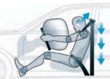
► **FRONT SEAT-BELT PRETENSIONER WITH FORCE LIMITER.** IN THE EVENT OF A COLLISION, THE PRETENSIONER TIGHTENS ANY EXTRA SLACK IN THE SEAT BELT, WHILE THE FORCE LIMITER LETS OUT THE APPROPRIATE AMOUNT OF SLACK WITHIN A FRACTION OF A SECOND AFTERWARDS TO REDUCE STRAIN ON FRONT OCCUPANTS.
