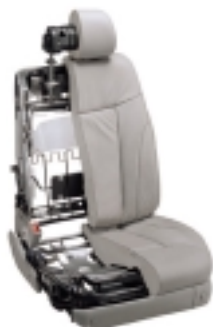
>> 8 way Power Seat (Sliding, Reclining and Seat Height Adjustable)
