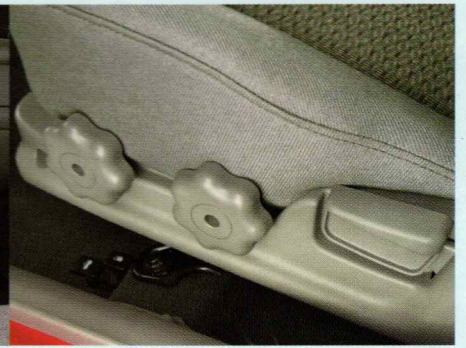
Driver's seat height adjuster in Rio RS and LS
