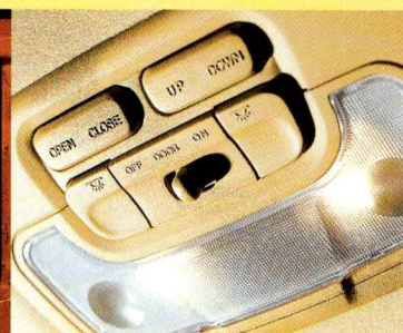
Roof console with map lights and sunroof control
