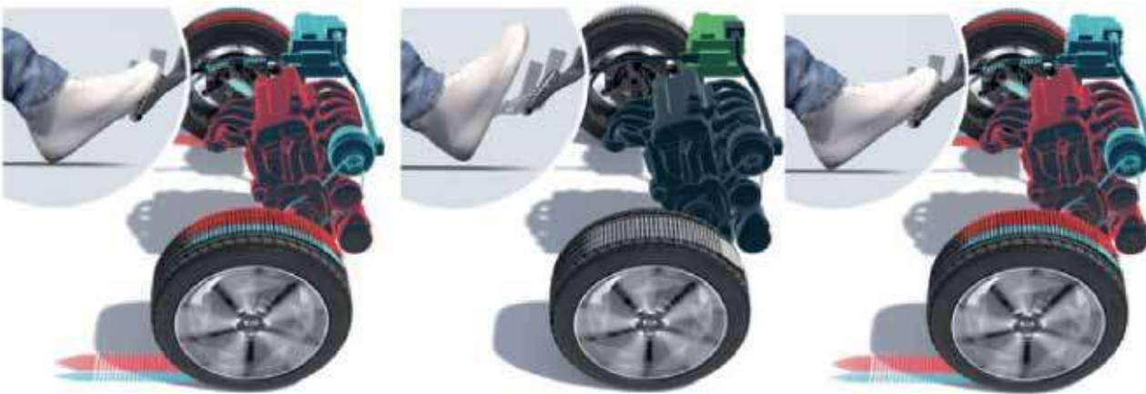
Simplified visual representation of the Mild Hybrid iMT sailing operation.
