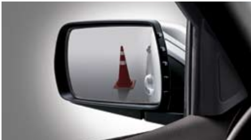
Outside mirror (available with IMS) When the gearbox is in the 'R' position, the outside mirror automatically adjusts downward to provide unobstructed rear sight lines for added safety.
