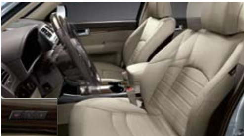
IMS (Integrated Memory Seat) system Mohave electronically records settings for two different driver seating positions and automatically readjusts the driver's seat, outside mirrors and steering wheel. The steering wheel selects the most recent position when the engine start button is activated, and the seat moves back 5 centimeters when 'P' gear is selected to enable easy vehicle access.
