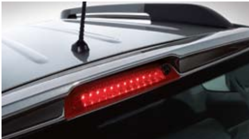
High-mounted stop lamp Studies have shown that a high-mounted stop light, like the Mohave's high-mounted LED stop light located on the tailgate, is a major contributor to road safety, making your intentions to slow down clearer to other road users.
