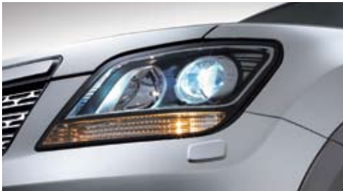
HID projection headlamps HID headlamps provide more intense, longer-lasting light for a better view of the road for the driver, and a better view of the Mohave by other motorists.
