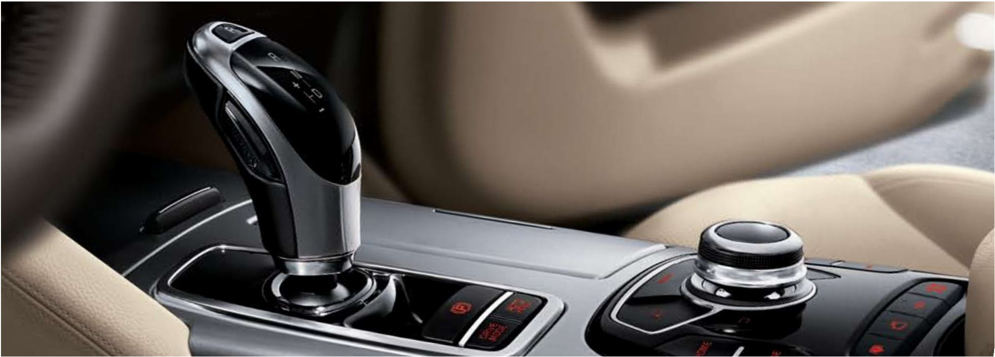
SBW (Shift-By-Wire) Electronic Gear Knob Kia Quoris features innovative SBW (shift-by-wire) technology, which removes any mechanical link between the gear selector and the gearbox. Together with a sensitive joystick control that delivers fast, smooth gear changes, SBW technology helps save space and weight while reducing engine noise in the cabin.
