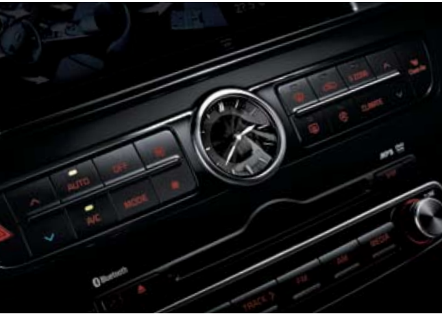
Three Zone, Full Auto Temperature Control For ultimate comfort and convenience, individual settings and thermostats for both driver and front seat passenger as well as the rear seating area enable customized climate control according to preferences.
