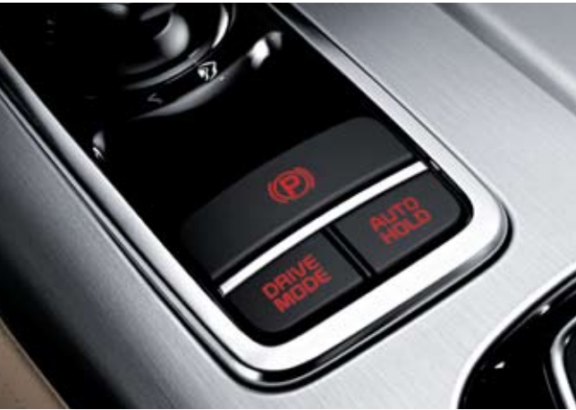
Auto Hold Switch This innovative feature automatically maintains the vehicle in standstill after the driver brings the vehicle to a complete stop by foot brake, then releases by acceleration. You no longer have to keep your foot on the brake pedal to prevent the vehicle from rolling away accidentally when stopped on an incline or caught in slow traffic.
