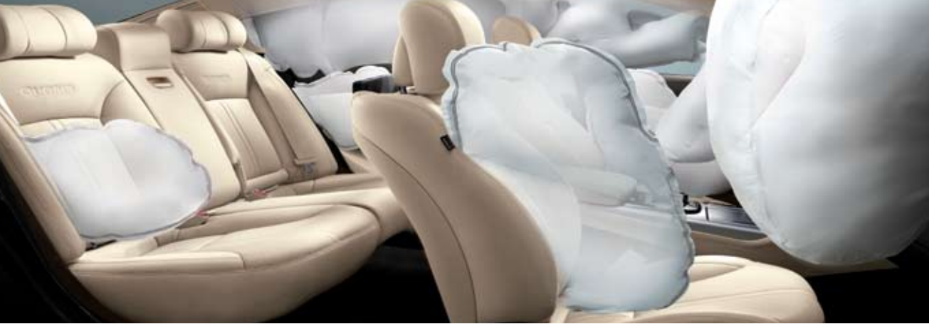
Advanced 9-Airbag System Kia Quoris provides an exceptional level of protection from the impact of collisions for all occupants thanks to dual front, twin front seat side and full-length curtain airbags, plus twin rear seat side airbags and a driver's knee airbag. An intelligent airbag mechanism ensures deployment at an appropriate pressure based on the intensity of the collision to prevent excess injury.
