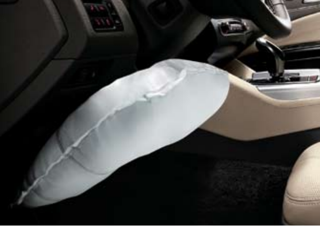
Driver's Knee Airbag In the event of a crash, the driver's knee airbag deploys to prevent injury to the lower body by offering extra protection for the driver's legs and feet from impact with the steering column and instrument panel.
