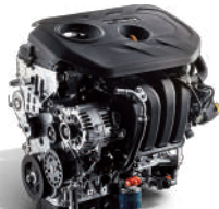
Nu 2.0 GDI 165 Ps/6,200 rpm 203 N·m/4,700 rpm + 6挡手自一体变速器
