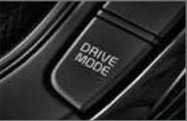
Drive Mode Select (DMS) DMS lets you choose Comfort or Eco mode to suit your preferences and driving conditions, or a new Smart mode, which switches between these two modes based on how you drive. *Sports mode is initiated when you move gear level to the Ds.
