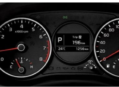
**2.6-inch mono-LCD** Get tyre pressure alerts and other essential vehicle and trip information at a glance with the mono LCD located between the instrument dials.
