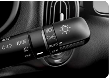
**Auto Light Control** Set the stalk ring to 'Auto' and the front and rear lights will turn on or off automatically depending on lighting conditions.
