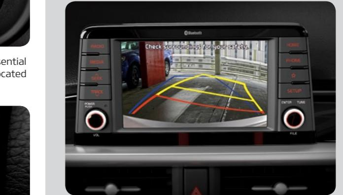
**Rear-view camera with graphic guidelines** Using a waterproof rear camera and the 7-inch dash display, the rearview camera projects graphic guidelines onto the image to recommend a path as the driver reverses. S-MART models only.
