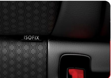
**ISO FIX Child Seat Anchor** The all-new Picanto is equipped with the ISO Fix points to secure child car seats quickly and safely without using seat belts.
