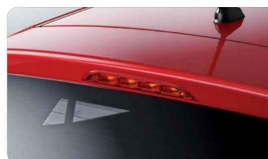
**High-mounted Stop Lamp** Located on the subtle spoiler above the rear window, the lamp safely alerts drivers behind you when you're braking.
