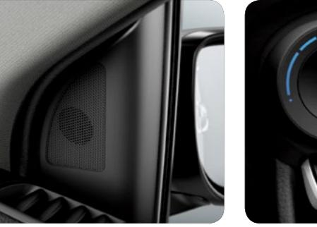
**Tweeters** Tweeter speakers at each end of the dash help bring out the high frequencies of the audio signal.
