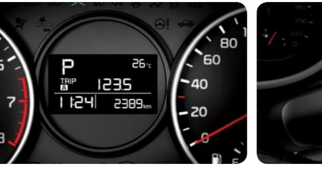
**Segmented Cluster LCD** A segmented cluster between the instrument dials keeps vital information front-and-center.
