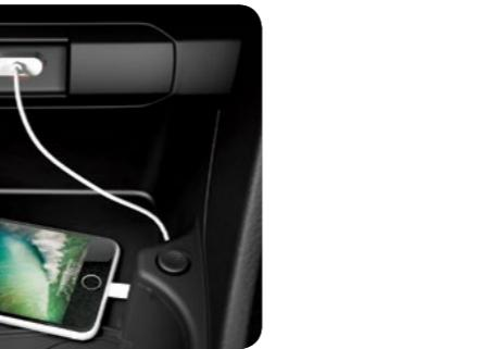
**AUX and USB Ports** Connect audio players and mobile devices via USB or mini-RCA cables for instant playback.
