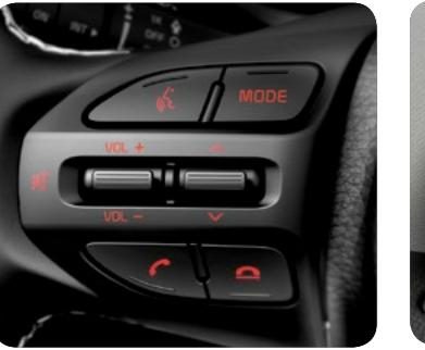
**Audio Remote Controls** Buttons mounted on the steering wheel let you adjust audio functions while your eyes stay on the road.
