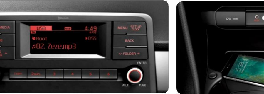
**Audio System** The optional five-speaker 3.0 audio system with RDS includes a monochrome TFT LCD screen. In addition to radio, it offers connectivity with portable devices through its AUX and USB inputs.
