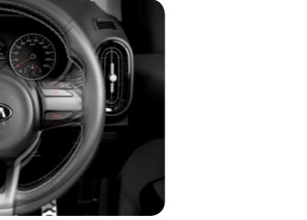
**MDPS with Tilt Steering Wheel** Motor-driven power steering simplifies turning, while a tilt steering column lets you find the most comfortable driving position.
