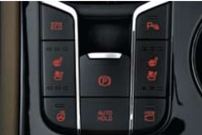
Electronic parking brake (EPB) Engage the parking brake simply by pressing a button and take all of the guesswork out of knowing whether it's properly engaged or not.
