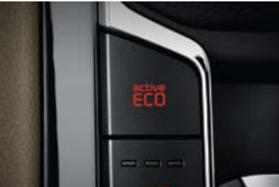
Active eco system The engine, transmission and air conditioner output are automatically controlled to achieve optimal fuel efficiency.
