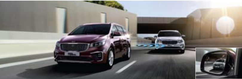
Blind-Spot Collision Warning (BCW) The system uses radar sensors to monitor approaching vehicles from the rear in the lanes flanking the driver. If a vehicle is detected, a visual alert appears on the sideview mirrors.
