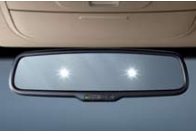
ECM rear view mirror This smart feature dims the rear view mirror automatically in response to trailing headlights for added safety when driving at night.
