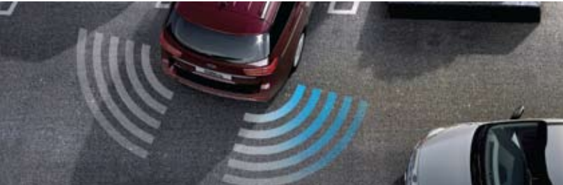
Rear Cross-Traffic Collision Warning (RCCW) When backing out of a parking spot or driveway, the system warns the driver if it detects any cross traffic in the lane the vehicle is entering.
