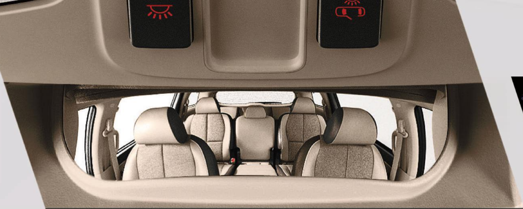
Conversation Mirror Looking over your shoulder while driving can be dangerous. Talk to rear-seat passengers without turning your head.
