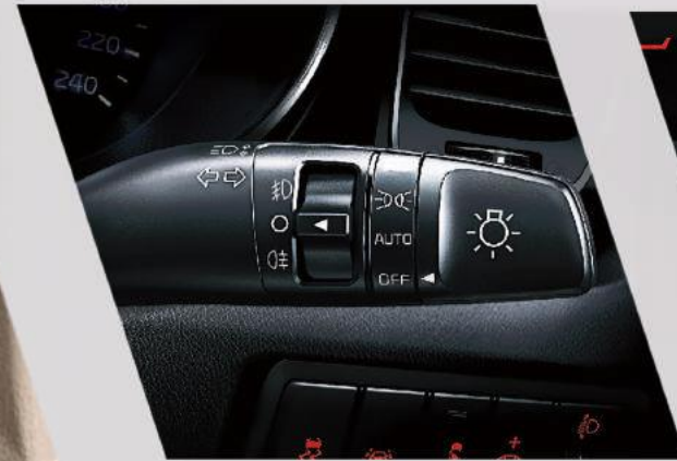
Auto Light Control The Grand Carnival's headlamps automatically switch on or off, depending on exterior light levels to make driving more convenient.
