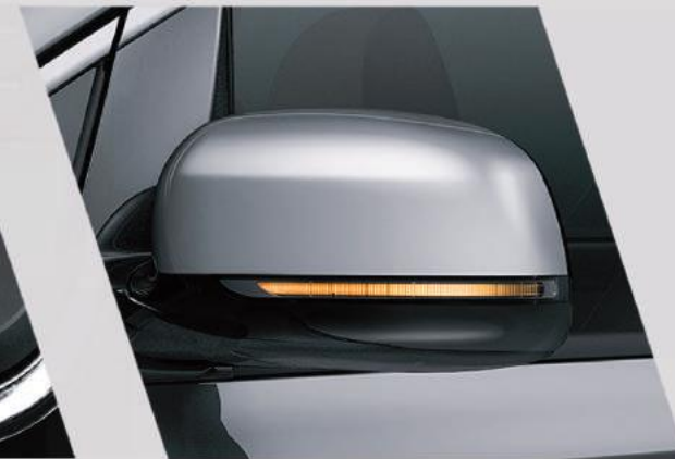
LED Side Repeaters and Auto Folding Mirrors The exterior side mirrors are heated and fold away automatically, for added convenience. They also incorporate LED side repeaters for a perfect fusion of function and form.
