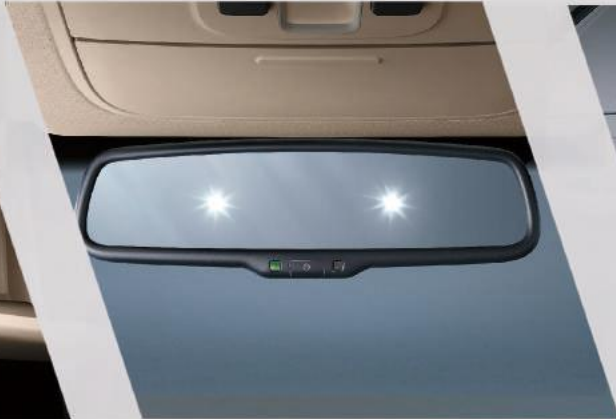
ECM Rear View Mirror The rear-view mirror automatically dims the headlights of trailing vehicles for added safety when driving at night.
