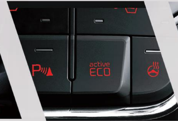
Active Eco System The Grand Carnival's engine, transmission and air conditioner output are all centrally controlled for optimal fuel efficiency.
