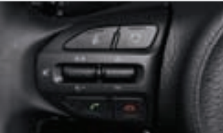
Steering wheel audio remote control Adjust audio settings using just your thumb, for enhanced driving safety.
