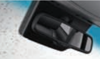
Rain sensor The rain sensor detects raindrops on the windshield and activates the wipers when a coverage threshold is met.
