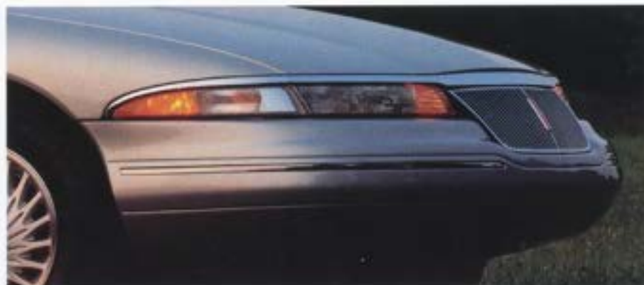
The front end is built for durability: Five-mph bumpers are made of resilient foam covered with plastic. Polycarbonate headlamp lenses resist breakage.
