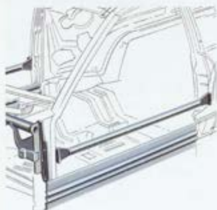
Door beams are made of ultra-high-strength, tubular steel.
