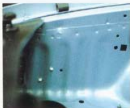
Convolutions stamped into the unitbody are intended to help the body absorb impact forces in a controlled manner.
