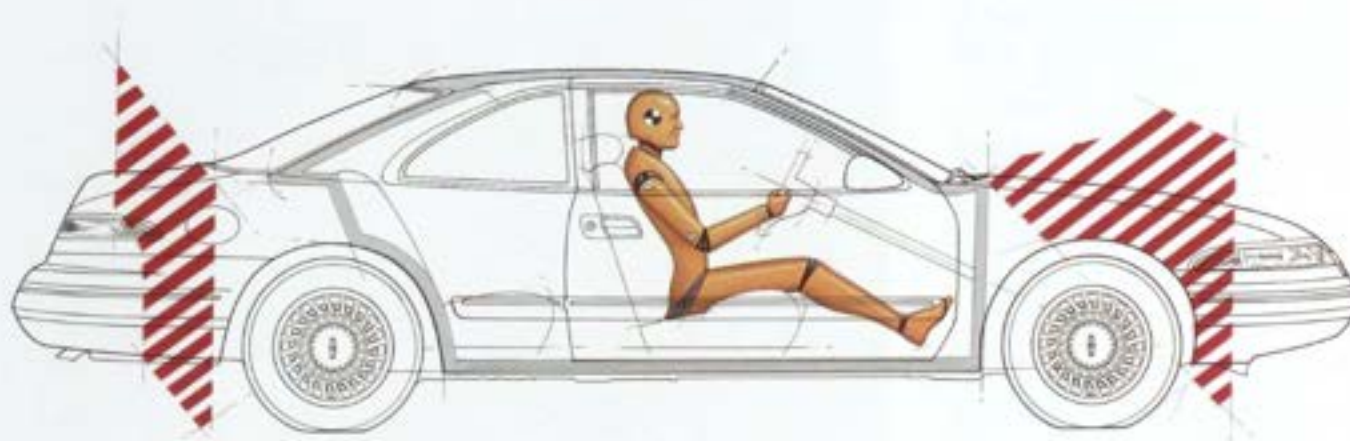
Crush zones in the front and rear of the car (shaded areas) absorb some impact energy in a collision, so it is not passed on to the occupants in the cabin.
