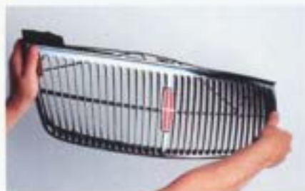
The soft chrome grille, made of indium bonded to thermoplastic urethane, resists damage caused by twisting or impact.
