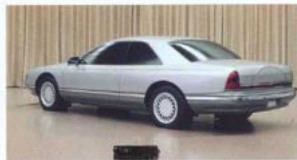
Scale models, like those shown above, were used to test design ideas during the early phases of the Mark VIII's development.
