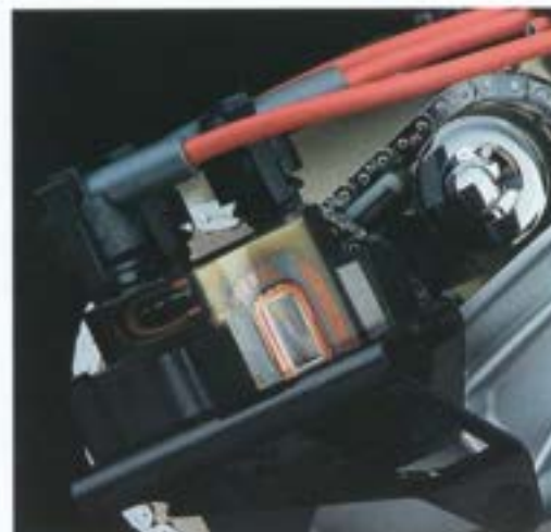
Electronically controlled coils deliver ignition spark, without a distributor.
