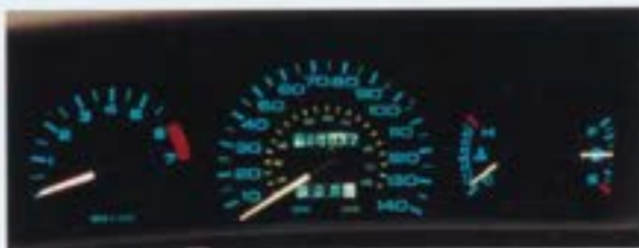
The Mark VIII's analog instrumentation shows information clearly and quickly, while indicating rate of change.
