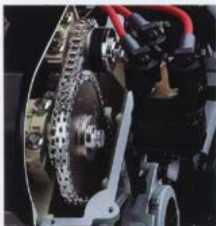
The chains that drive the camshafts are durable and operate quietly.
