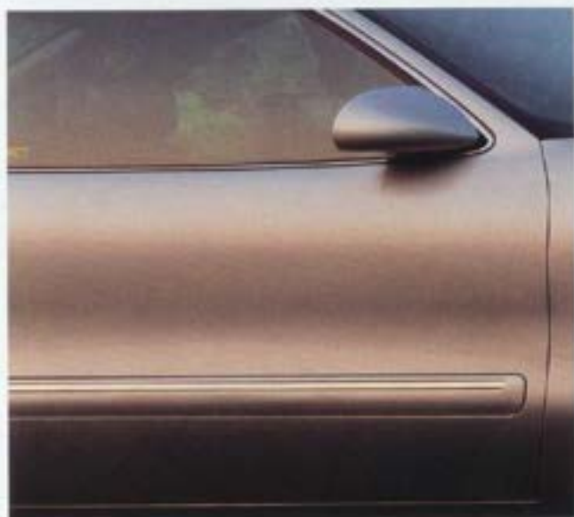
Protective moldings mount in recesses stamped into the door and quarter-panel sheet metal. Aerodynamically shaped mirror housings reduce wind resistance.
