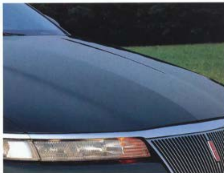
The sheet-molded-compound (SMC) hood is lightweight and cannot rust.
