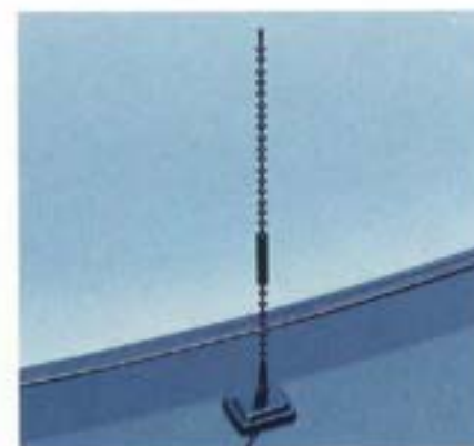
The available cellular telephone's antenna was designed to eliminate hum at road speed.
