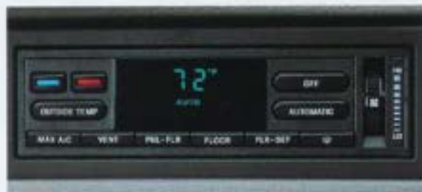
Above: The temperature-control panel is easy to understand and to operate.
