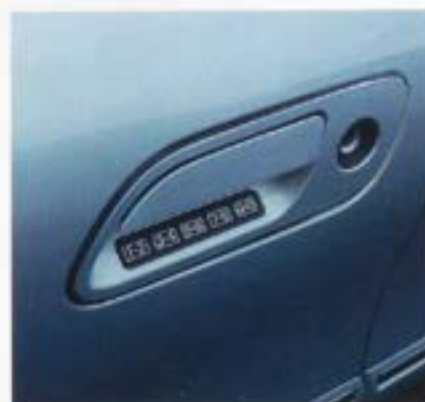
Top: The remote keyless entry transmitter locks or unlocks the driver's door or trunk from up to 33 feet. Above: A five-digit access code unlocks the doors and the trunk.
