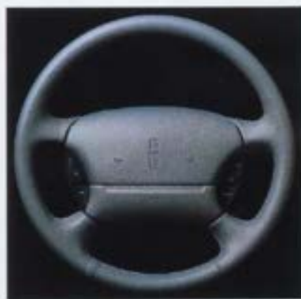
The steering wheel tilts for driver comfort and clear visibility of the instrument panel.
