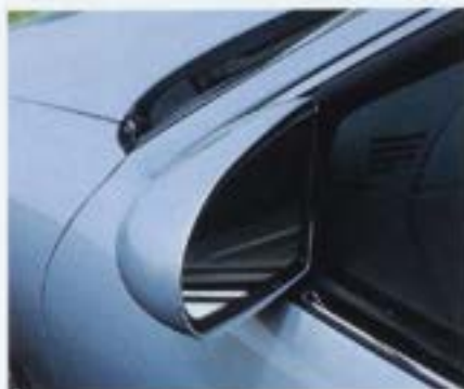
Electrically heated exterior mirrors provide a clear view in adverse driving conditions.
