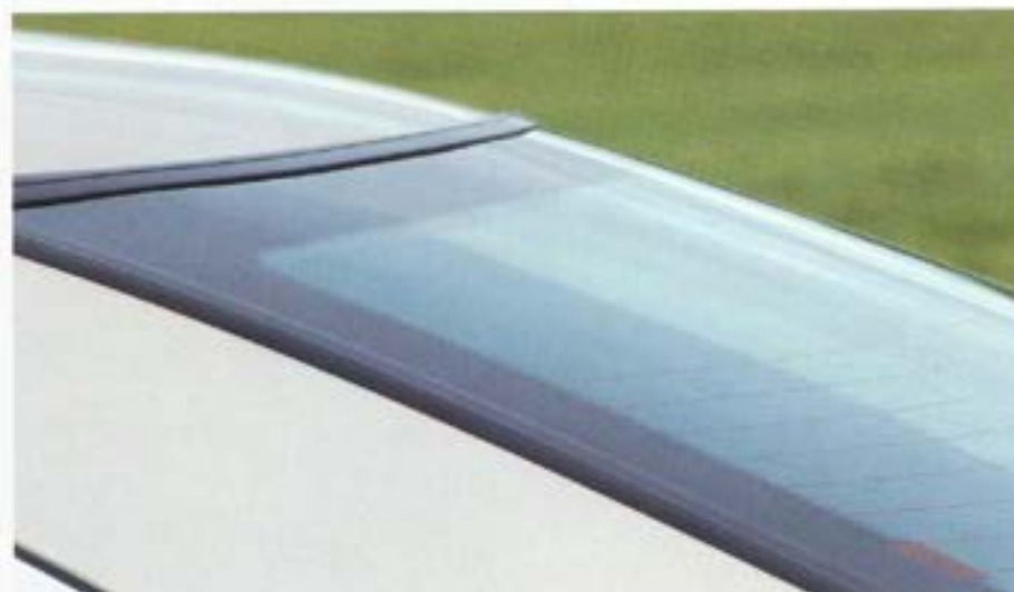
The one-piece molding is bonded to the rear window during manufacturing, and it is mounted to the body at zero tolerance, for a perfect fit and leak resistance.
