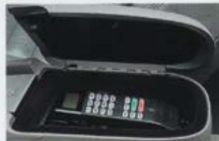
Top: The optional voice-activated cellular telephone is controlled by a button on the A-pillar, where the microphone is located.
