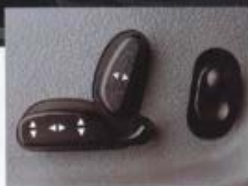
Switches for each of the front seats (inset) offer six-way, power control.
