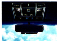
Overhead console features map lights, warning lamps, an electronic compass and an outside temperature display.
