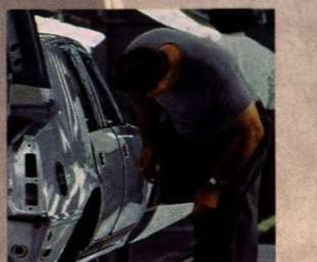
An inspector goes over a randomly selected vehicle inch-by-inch to check on fit and finish.
