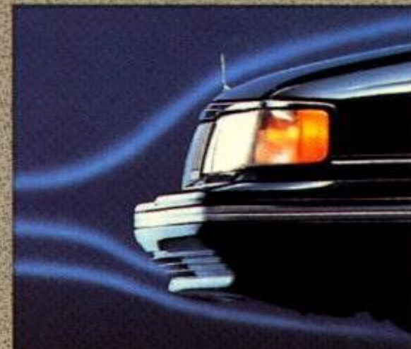
Extensive wind-tunnel testing led to Continental's favourable 0.35 drag coefficient.
