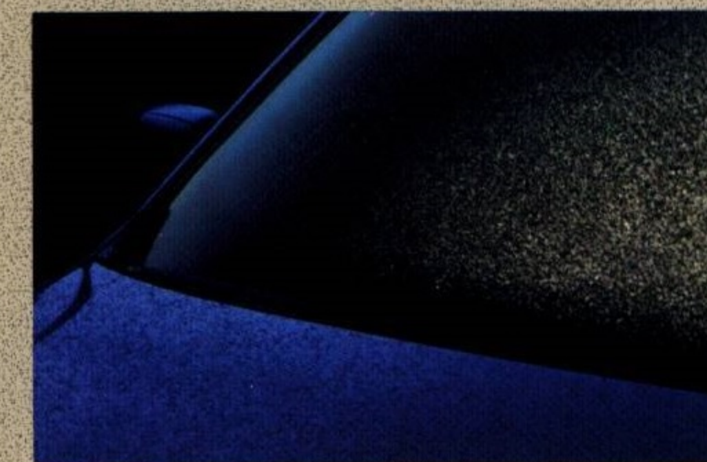
Continental's optional Insta-Clear™ windshield uses a transparent metallic coating to spread heat over the windshield's entire surface.
