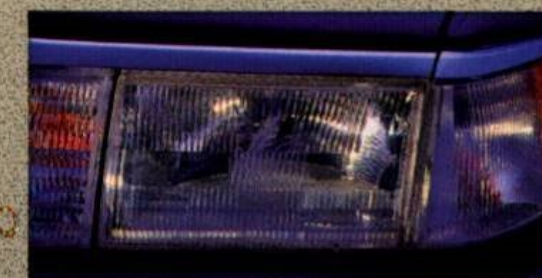
Aerodynamic headlamps have impact-resistant polycarbonate lenses.
